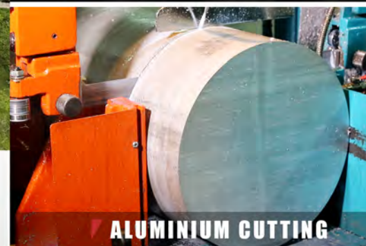
BC Forged Wheels are using aerospace grade Forged 6061-T6 Aluminium, then CNC machined in highest precision and perfection, in order to achieve the best balance for strength and light weight.
